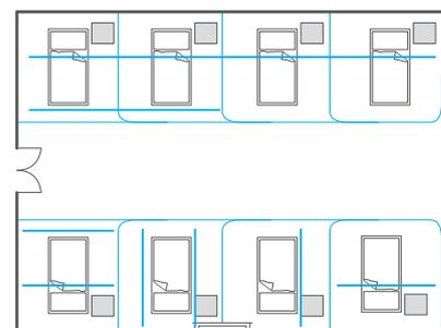
There are several alternatives for IV200 track positions. The most commonly used layout is a track parallel to the back wall and 1m out from it. A continuous track is then possible over the line of beds, assuming an unobstructed ceiling. A second track may be positioned across the foot of the beds if required. Another alternative is a track running parallel to the bed. This gives IV provision at both the head and the foot of the bed, and also allows stacking of carriers against a wall.
