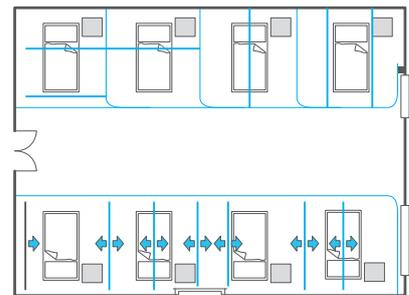
IV400 lends itself to many configurations within a hospital bed cubicle. The most common configurations of fixed track are shown here, but the specifier should take account of medical factors such as levels of usage, and the possible need of secondary IV provision at the foot of the bed.
